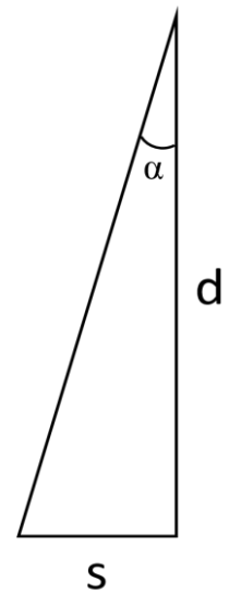
Figure 2: Use trigonometry to determine the angular separation of the stars at the point they could be resolved.
